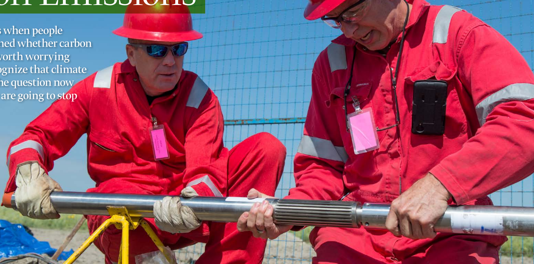
Workers prepare a borehole gravity logging tool for deployment down the Aquistore injection well. One of many technologies in use at the site. Photo: Brian Zinchuk
